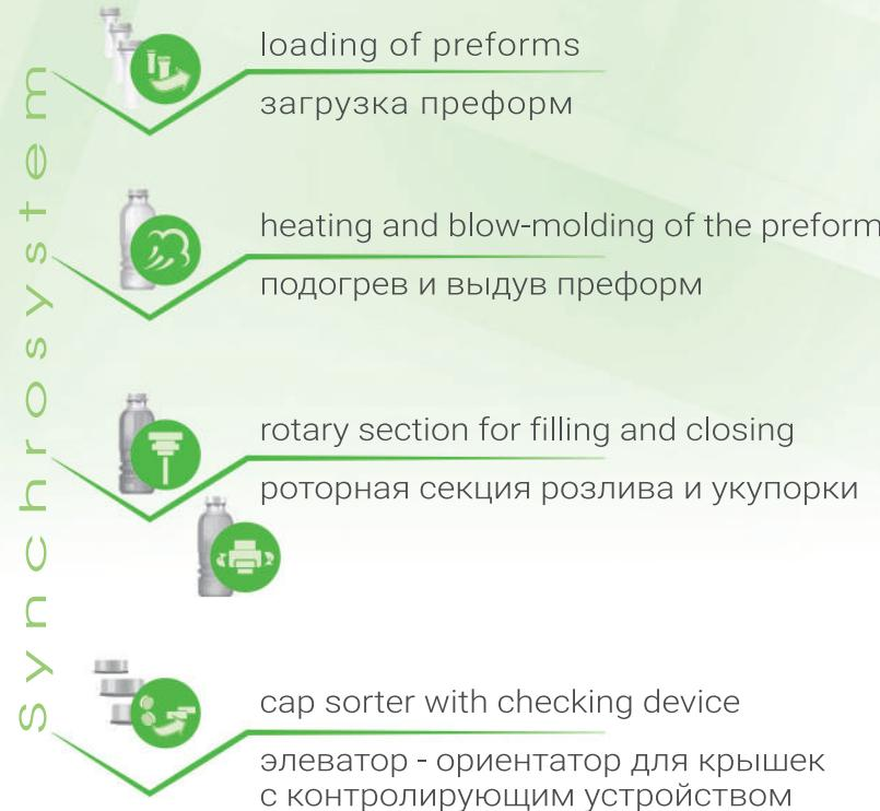
Integrated automated monitoring system for preforms and caps supply, synchronization, filling and closing by a dual operating system.
